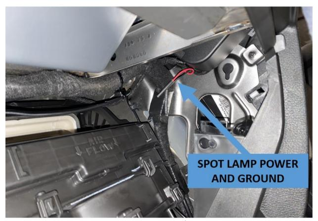
Figure 25: Passenger side spot lamp blunt cut circuits (view with glove box removed, looking from center of vehicle towards outboard right side)
