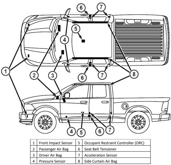
**Figure 26: Occupant Restraint System Components**
