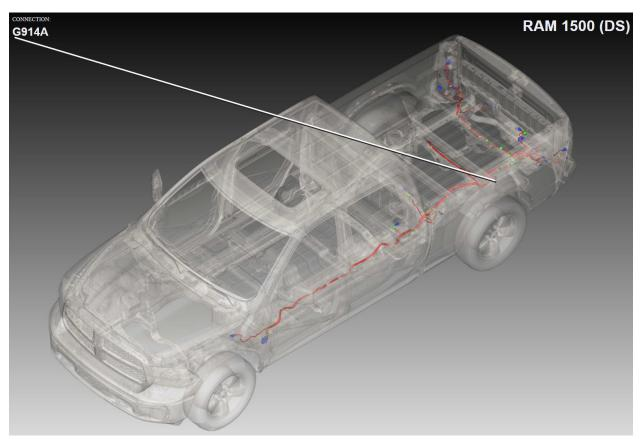
Figure 8: Grounding location at rear frame
