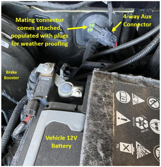
Figure 13: 4-way underhood Aux connector
