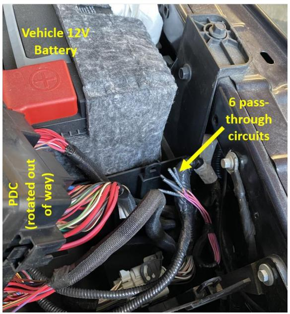
Figure 9: Pass-through circuits underhood
