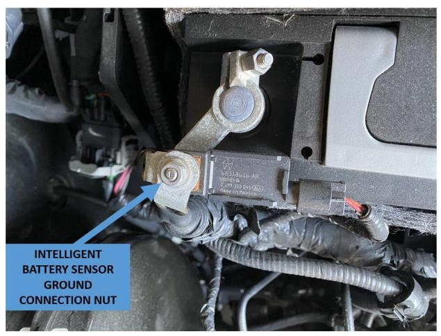
Figure 36: Intelligent Battery Sensor
