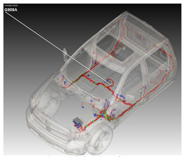
Figure 7: Grounding location between front seats
