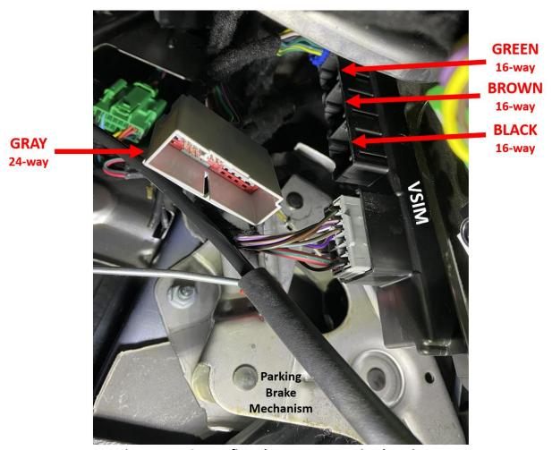
Figure 17: VSIM upfitter harness connection locations
