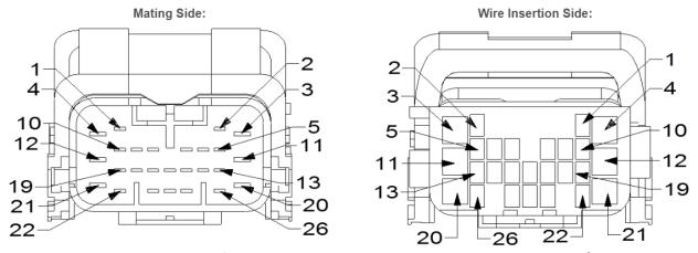
Note: This is the view of the vehicle harness connector, not the mating jumper/pigtail
